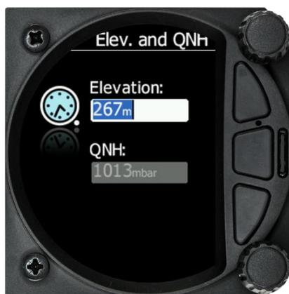
The user has to set either the Elevation or the QNH with the lower rotary button. After pressing the lower rotary button the user can switch between the Elevation and QNH dialogues. As soon as the settings are set the middle button must be pressed in order to proceed.
