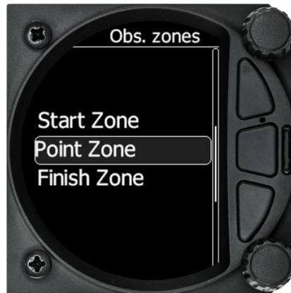
The Start, Turn point and Finish zone can be configured separately although the setup is very similar.
