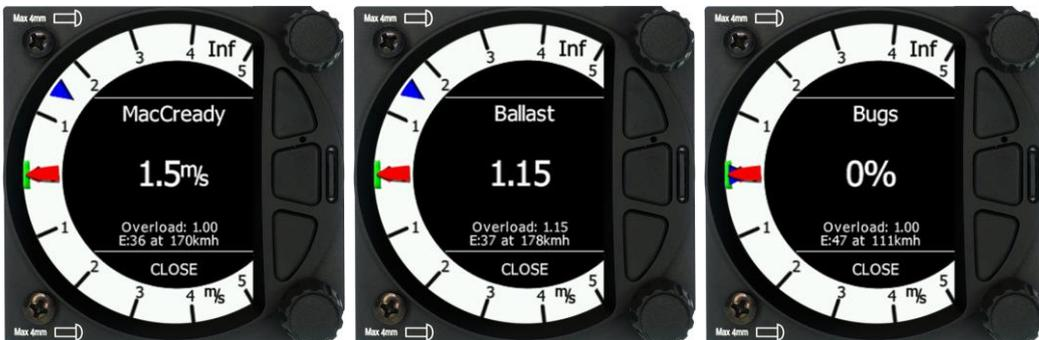
Rotate the bottom knob to modify any setting. Next check the safety altitude (height above destination, arrival altitude) setting. Refer to Section 5.7.1.2 to find how to define the safety altitude.
