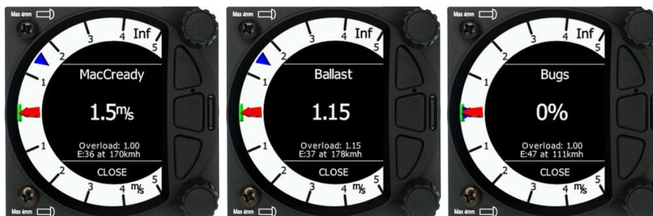
To change the MacCready value press the bottom rotary knob and press on MC/BAL. A short press of the lower rotary knob moves from MacCready to the Ballast box and pressing the lower rotary knob again will open the Bugs box. If no action is performed within 3 seconds, the box will close or you can also press CLOSE anytime (lower push button).
